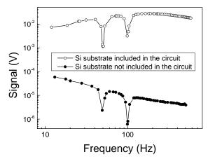
Fig. 3 Frequency dependence of the pyroelectric signal measured with and without the Si substrate included in the measurement circuit.
