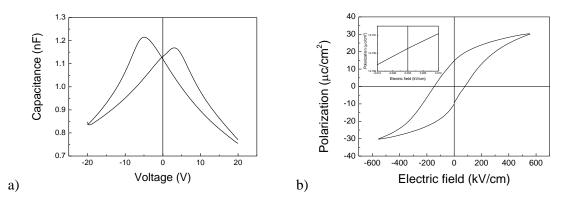
Fig. 5 a) the C-V characteristic of the PZT capacitor used as pyroelectric element on Pt/Si substrate; b) the hysteresis loop obtained for a PZT film deposited on Pt/Si substrate. The inset shows the polarization variation at low electric fields, around zero volts/cm.
