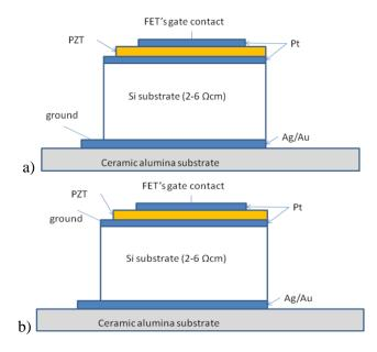
Fig. 2 a) connection with the Si substrate included in the measurement circuit, considering the entire Pt/Si/Ag/Au stack as bottom electrode for the PZT film; b) connection without the Si substrate included in the measurement circuit (ground contact on the Pt layer deposited on Si, gate contact on the top Pt electrode).
