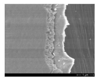
Fig. 1 SEM photograph of the PZT film deposited by sol-gel on Pt covered Si wafer.
